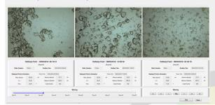
up to 6 sensors in real time. Connected to the plant PLCs and DCS it offers great potential for a tighter control of the crystallization process.
