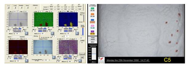
Over time the on-line system became so robust in its performance and the operators were so confident in its capability to manage the sugar colour that they requested an upgrade to the controller program. The change requested was to amend the controller logic to alter the wash timers by only 0.1 second each time, rather than the 1 second changes that was initially used. This further refined the overall performance and reduced over compensation to changes in colour by the controller logic.
