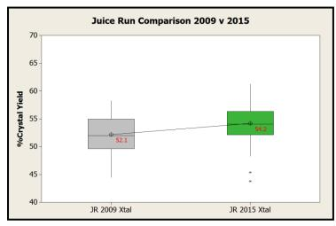
Graph 9 – Reduction in "Out of Spec" white sugar produced by the white centrifuges, before and after the development of the online colour system
