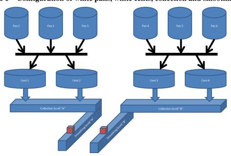
The aim of the installation was to monitor every batch of sugar discharged from each of the four white centrifuges, as it passed through the smoothing scrolls. The output from the colour
